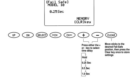
**Note:** If Fail-Safe does not appear on your LCD, it is because you are transmitting in PPM. Fail-Safe is not applicable in the PPM mode. Refer to the Modulation Mode Selection Section for more information.
