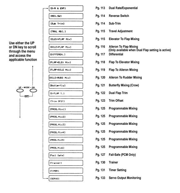
To enter the List Mode, press the DN and SEL keys simultaneously. From this display, pressing the UP and DN keys simultaneously will move the system from the list mode to the
