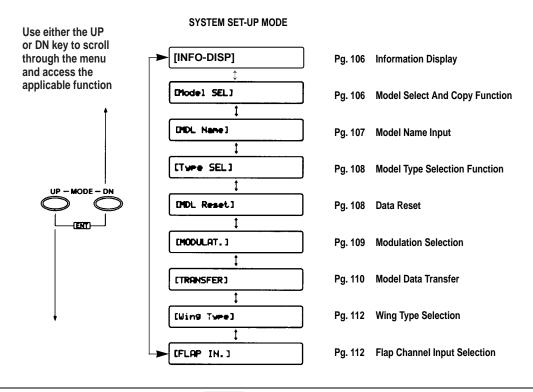
From Normal Display, press the UP and DN keys simultaneously to enter the Function Mode. In this mode, by using the UP or DN keys, the desired functions can be selected. When channel selection or an additional function change is desired, use the CH keys or SEL key. For example, Dual Rate Function is selected and the elevator channel is displayed by pressing the UP key once; the function is changed to the next mode, Reverse Switch, but the channel is still displayed as elevator.
