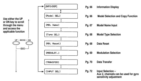
From Normal Display, press the UP and DN keys simultaneously to enter the Function Mode. In this mode, by using the UP or DN keys, the desired functions can be selected. When channel selection or an additional function change is desired, use the CH keys or Select key. For example, Dual Rate Function is selected and the elevator channel is displayed by pressing the UP key once; the function is changed to the next mode, Reverse Switch, but the channel is still displayed as elevator.
