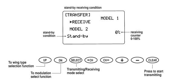
The purpose of Wing Mixing or Wing Type Function is to eliminate mechanical or programmable mixes that would otherwise be necessary for the proper flight of certain styles of aircraft. There are three wing types from which to choose; select the one that best suits your R/C aircraft. They are as follows: Normal, flaperon, and elevon (delta). Each of the wing type selections will be covered in a separate section.
