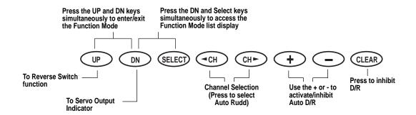
The Reverse switch is an electronic means of reversing the throw (direction) of a given channel (servo). All eight channels of the XP8103 offer reversible servo direction. This will ease set-up during servo installation in your aircraft.
