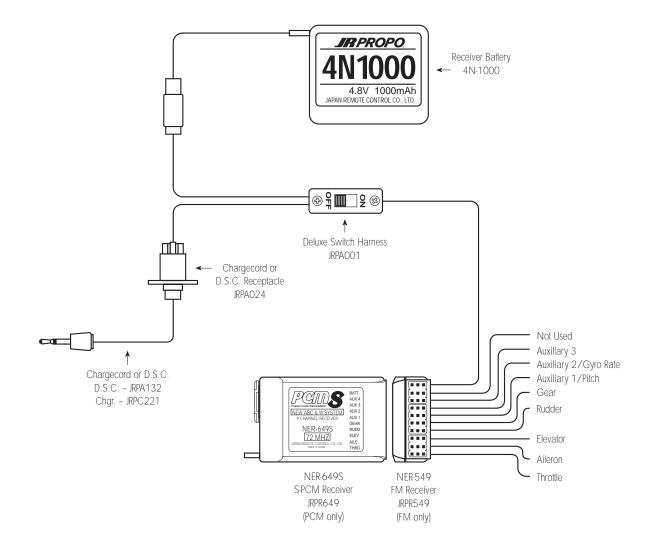
Connect the gyro to the axis to be controlled (commonly rudder channel) per the illustration below.
