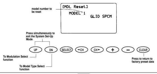
The Modulation Selection Function enables your XP8103 to transmit to a variety of JR receivers that are already, or may soon be, in existence. You can select from either S-PCM or Z-PCM mode, depending on the Central Processing Unit within your receiver, or from PPM (Pulse Position Modulation—FM). Refer to the receiver compatibility chart for the correct modulation.
