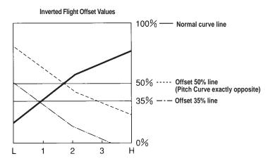
As shown above, when the offset value is set for 50%, the inverted flight pitch curve is exactly opposite from the normal pitch curve settings. If the offset is adjusted to a lesser value, say
