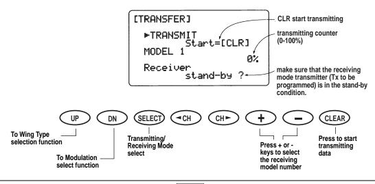
When there is a data receiving failure during transmitting, the counter will stop. At this time, press the CLR key to stop the receiving condition. Check to be sure the receiving counter is operating normally and ended with 100%. If there is any failure
