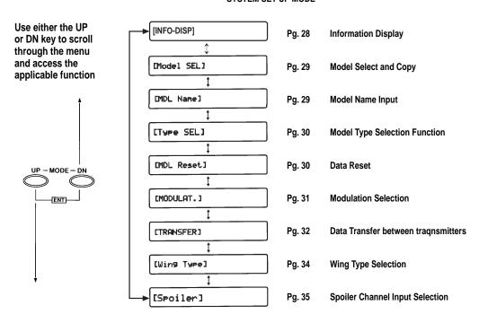
From Normal Display, press the UP and DN keys simultaneously to enter the Function Mode. In this mode, by using the UP or DN keys, the desired functions can be selected. When channel selection or an additional function change is desired, use the CH keys or SEL key. For example, Dual Rate Function is selected and the elevator channel is displayed by pressing the UP key once; the function is changed to the next mode, Reverse Switch, but the channel is still displayed as elevator.
