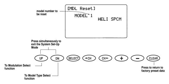
TThe Modulation Selection Function enables your XP8103 to transmit to a variety of JR receivers that are already, or may soon be, in existence. You can select from either S-PCM or Z-PCM mode, depending on the Central Processing Unit within your receiver, or from PPM (Pulse Position Modulation—FM). Refer to the receiver compatibility chart for the correct modulation.
