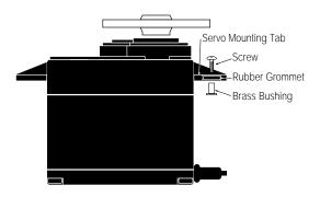
2. The servos should be mounted using rubber grommets and brass bushings to isolate them from vibration. Do not over-tighten the mounting screws — this will negate the vibration absorption effect of the rubber grommets. The diagram at left will assist you in properly mounting your servo.
