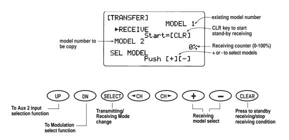
When the receiving counter is stopped or you see ERROR indicated, check the DSC cord connections or trainer cord conditions and try again. When data has been received correctly, you will see [End ok] display. Be sure that the receiving mode transmitter is in stand-by condition first. Then on the transmitting transmitter press the CLR key to start transmitting.
