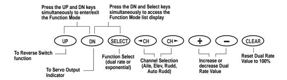
When the Automatic Dual Rate function is activated (ACT), when switching the Flight Mode switch to Stunt 1 or Stunt 2, or when switching the throttle hold switch ON, the Aileron, Elevator, and Rudder channel dual rate values can be switched to the values set for dual rate position #1. Once the Automatic Dual Rate function is selected for a flight mode (1, 2, and/or hold), AUTO will appear on the D/R screen when the flight mode switch is moved to the selected position.
