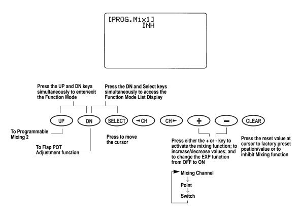
The XP8103 offers six (6) programmable mixes to be used for a number of different purposes. The functions allows mixing any one channel to any other channel.
