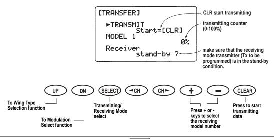
When there is a data receiving failure during transmitting, the counter will stop. At this time, press the CLR key to stop the receiving condition. Check to be sure the receiving counter is operating normally and ended with 100%. If there is any failure of transferring, the display will appear as follows:
