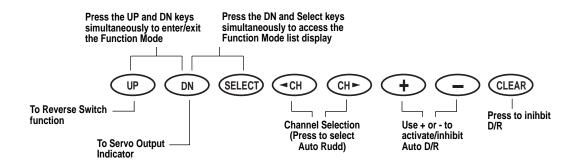
The Reverse Switch is an electronic means of reversing the throw (direction) of a given channel (servo). All eight channels of the XP8103 offer reversible servo direction. This will ease set-up during servo installation in your aircraft.
