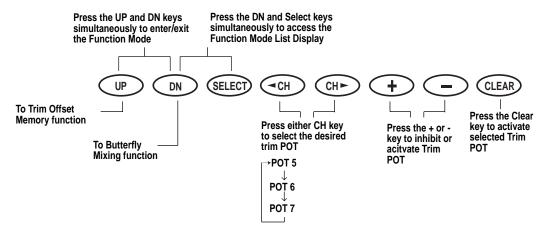
**Note:** Only POT 5 will appear on the LCD unless the Dual Flap Mixing Function is activated in the Wing Mixing Function. Refer to the Wing Mixing Function for more information on how to activate the Dual Flap Mixing Function.
