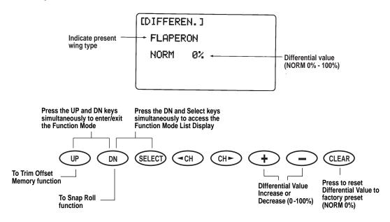
The Trim Offset Memory Function allows you to test fly your aircraft and correct for any built-in trim requirements. After you adjust the aileron, elevator and/or rudder trim levers during test flights, the trim levers are no longer in their center, or neutral, positions. The use of trim offset allows you to return them to their central or neutral positions without readjusting the linkages.
