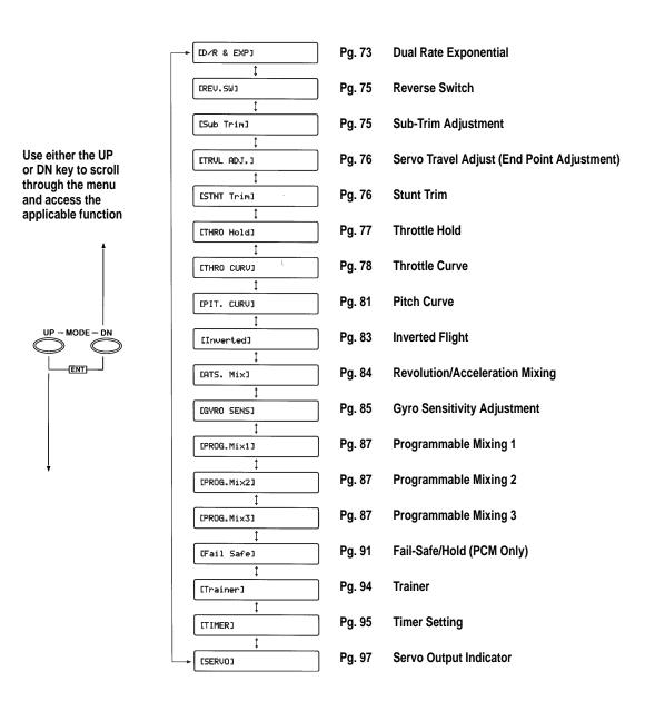
To enter the List Mode, press the DN and SEL keys simultaneously. From this display, pressing the UP and DN keys simultaneously will move the system from the list mode to the
