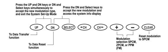
This function is used to transfer all existing memorized data for a model from one XP8103 transmitter to another XP8103 transmitter.
