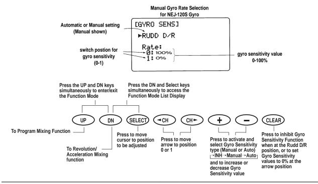
two pre-determined settings through the use of the flight mode switch. As different flight modes are selected (Normal, 1, 2, Hold), the Gyro's sensitivity rate will switch to the pre-determined compensation rate for each particular flight mode in use.
