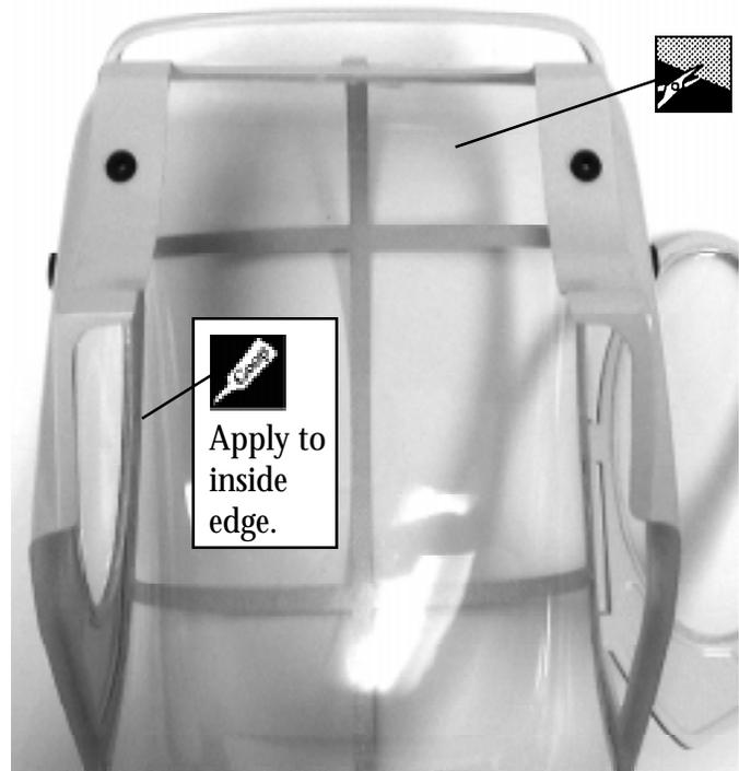
**Tip:** Use a small blade screw driver to apply the adhesive to the window/cabin joint. Attempting to apply the adhesive directly from the tube will likely result in runs on the exposed areas of the window.
