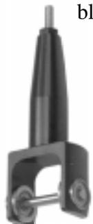
**Tip** On the 46SE kit the bellcrank needs to be modified as shown to avoid binding at high cyclic while inverted. Use a file to cut a bevel as shown.
