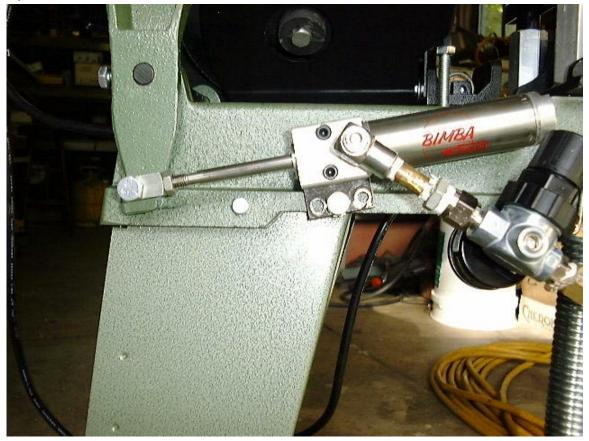
There has been some discussion of replacing the spring that controls the downward cutting force on the cheap  $4 \ge 6$  bandsaws sold by Harbor Freight and others. It has been suggested that a hydraulic cylinder with a flow control valve to keep the saw from coming down too fast would be a good replacements. I replaced the spring with an air cylinder and a flow control valve.
