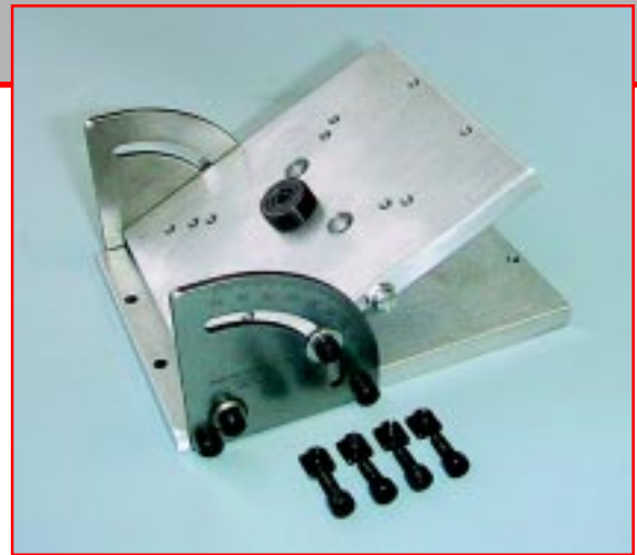
FIGURE 64—The tilting angle table makes many interesting setups possible on the mill. It also allows you to hold a part on an angle so it can be drilled or milled without taking your column out of alignment.
