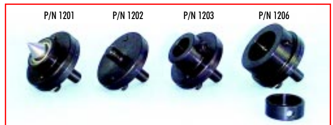
FIGURE 28—Adjustable tailstock tools make it possible to achieve "perfect" alignment between the headstock and the tool held in the tailstock. From left to right are the adjustable live center, adjustable drill chuck holder, adjustable custom tool holder and adjustable 1" die holder
