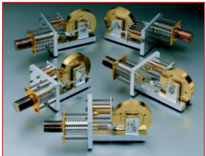
Project: Five identical Stirling hot air engines. Tim built this as his first project and made five of each part to improve his machining skills faster.
