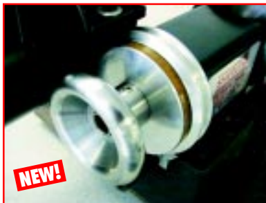
FIGURE 17 —The steel spindle handwheel makes it easier to control the spindle by hand.
