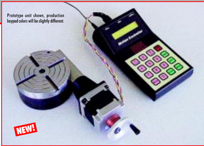
FIGURE 87 —For complex indexing jobs Sherline's 4" rotary table is the perfect platform for the application of CNC controls. Included is a programmable input unit that contains its own microprocessor, keypad and power supply.
