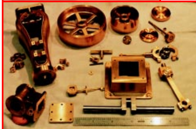
"Coke bottle" steam engine Chuck Sherwood, Naperville, IL Chuck took on quite a challenge to build this steam engine from a bronze casting kit as his first machining project. The top photo shows the completed engine, and the second photo shows the unassembled individual components. A ruler is used for size reference.
