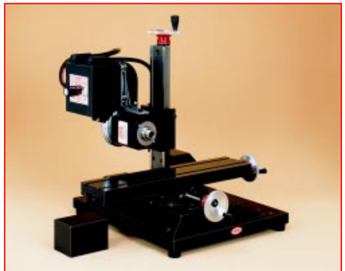
FIGURE 93 —The horizontal milling conversion allows the column of the vertical milling machine to be repositioned in various ways on a specially machined base in order to provide greater versatility in set-up and increase the machinable area of the parts being worked on. This set-up takes advantage of the long 9" X-axis travel. Another position 2-1/4" further from the table is useful for drilling operations. (Position "A".) Shown to the left of the milling conversion baseplate is the base of the Z-axis column, which has been cut off to allow a lower positioning of the headstock in relation to the table.
