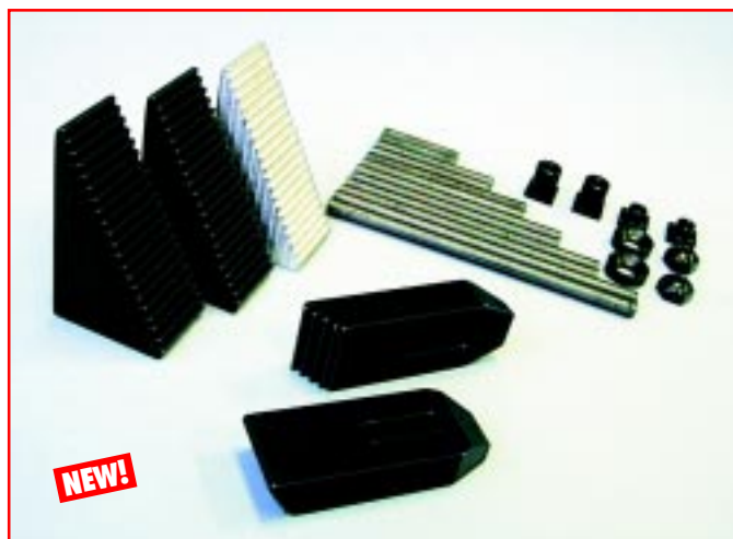
Figure 75—A step block set offers a quick and versatile way to clamp parts to the mill table.
