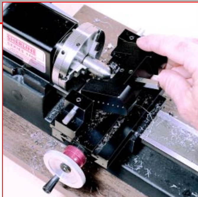
Figure 33 —The radius cutting attachment can cut a convex or concave radius. Unlike most lathe operations, the tool is moved up and down rather than horizontally.
