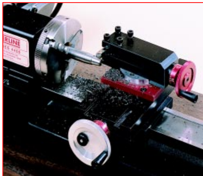
FIGURE 32 —The compound slide offers another way to cut tapers on a Sherline lathe.
