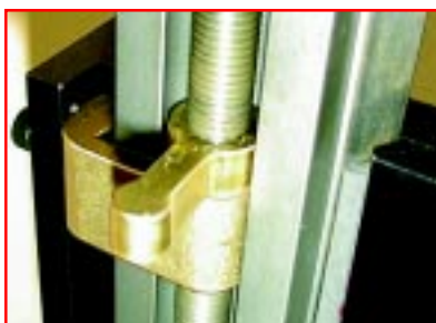
FIGURE 56—The saddle locking lever provides a very positive lock for the Z-axis and is standard on all new Sherline mills.
