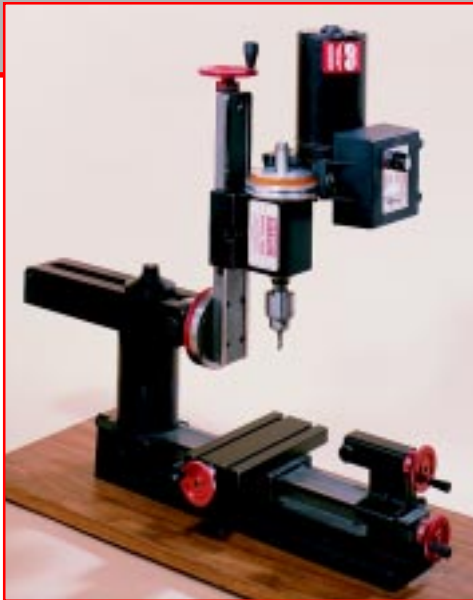
FIGURE 5—The new multi-direction vertical milling column opens up many new machining possibilities on the lathe by turning it into an 8-direction mill.
