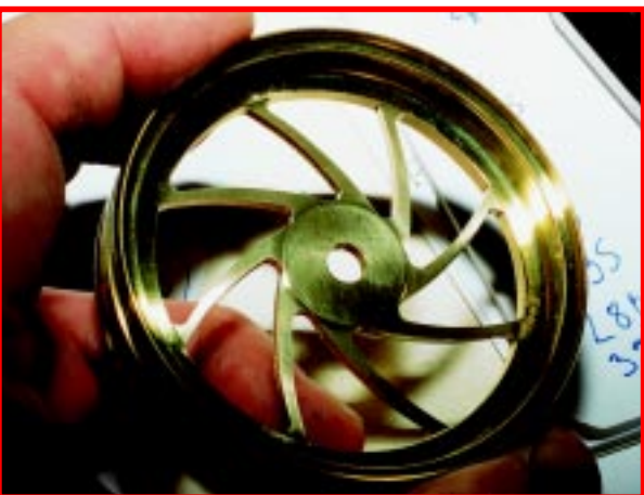
Custom brass wheel • Bob Breslauer Bob designed a clever double rotary table fixture to machine these curved spokes.
