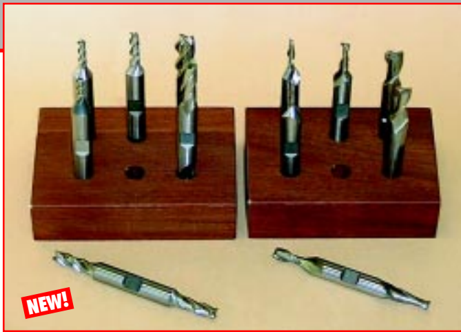
FIGURE 69 —Double-ended 3/8" end mills fit in the P/N 3079 end mill holder. They are available in a large variety of sizes and shapes. For strength and maximum rigidity, use the largest diameter cutter your job will allow.
