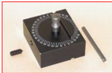
FIGURE 98—Mill headstock spacer block, precision-ground alignment key and set screw
