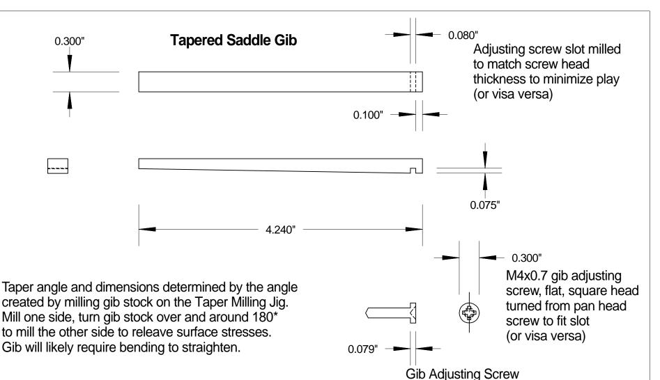
Taper thickness determined by the fit on your lathe. Make the tapered gib longer than needed (ie 6") and trim to fit tapered bracket assembled on carriage mounted on lathe bed.
